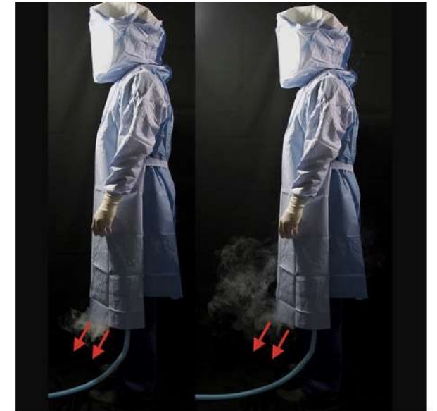
Figure 3. Air egress with the Flyte system and dedicated zippered suit.
